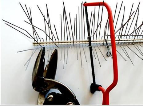
**6)** Cut spikes into smaller pieces to finish a row or to spike a small area. Spikes can be easily be cut using tin snips or a hacksaw.
